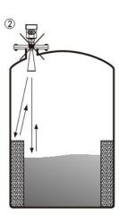
Take-over height requirements: The antenna must be inserted into the tank at least 10 mm away.
