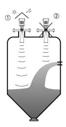
The meter cannot be installed in the middle of an arched or rounded tank top. In addition to generating indirect echoes, it is also affected by multiple echoes. Multiple echoes may be larger than the true echo signal threshold because multiple echoes can be concentrated through the top. So can't be installed in the center.
