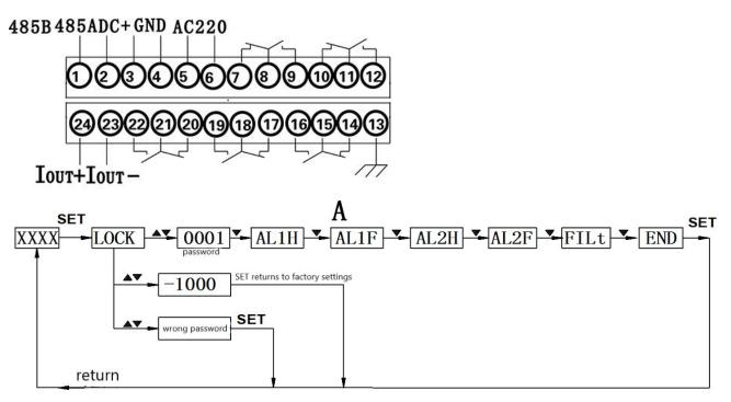
AL1H is the pull-in value of switch 1, AL1F is the release value of switch 1 AL2H is the pull-in value of switch 2, AL2F is the release value of switch 2 FILt this value is the display filter coefficient to prevent the display from jumping due to pressure fluctuation. The larger the filtering coefficient is, the more stable the display is, but the more lagged it is. 3 ~ 10 options
