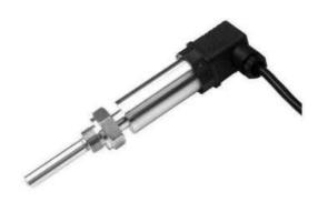
WMT180S Temperature Transmitter is a compact structure type which can be on-site installed to measure temperature and transmit corresponding signal. It consists of RTD and temperature transmitter chip that adopts two-wire output of  $4\sim20\text{mADC}$  or other user specified signals for transmission. It is widely used in automatic temperature measurement and control systems such as petroleum machinery, chemical machinery, pumps and compressors, electric power, boilers, and natural gas etc.
