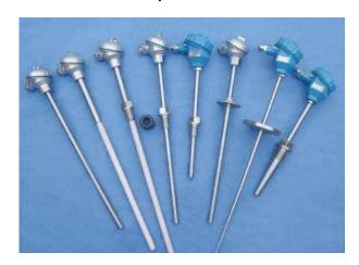
WMT180Y Temperature Transmitter is a kind of instrument which can be on-site installed to measure temperature and transmit corresponding signal. It consists of thermocouple or RTD and temperature transmitter module that adopts two-wire output of 4~20mADC or other user specified signals for transmission. It is extensively applied in the petroleum, chemistry industry, metallurgy, electric power, textile industry, food processing etc.
