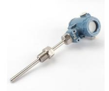
WMT180X Temperature Transmitter can be on-site installed to measure, display temperature and transmit corresponding signal to remote device. It consists of thermocouple or RTD, temperature transmitter and display module that adopts two-wire output of 4~ 20mADC or other user specified signals for transmission. It is extensively applied in the petroleum, chemistry industry, metallurgy, electric power, textile industry, food processing etc.
