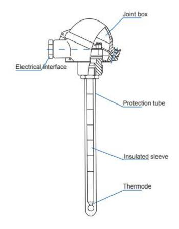
a. For the thermocouple more than 1m, the product of insulated resistance at normal temperature and its length is 100Mohms.m.
