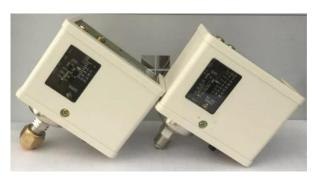
WM12020 universal pressure switch is a kind of pressure switch with ingenious structure and flexible use. It is equipped with bellows and mechanical mechanism. When pressure rises or falls, the corresponding mediation springs and ripples produce stretch or contraction displacement, and then push the switch through the lever action, cut off or switch on the control loop.
