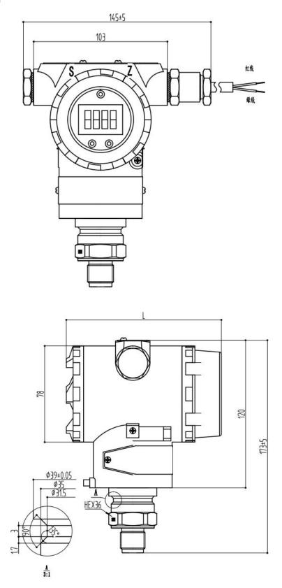
Note: With display L=126±5mm Without display L=108±5mm
