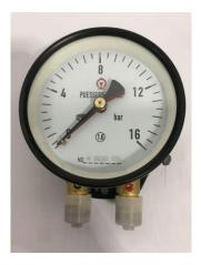
WYD-X Double Needle Duplex Pressure Gauge is mainly used for locomotive vehicles used to measure the pressure inside the hydraulic system or cylinder. It can also be used for non-corrosive, non-crystalline and solidification of the various media pressure measurement. The instrument can simultaneously measure two pressures that are the same or different (the difference between the two should not be greater than 1/3 of the upper limit of the scale range).
