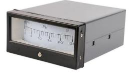
WYRC-X Rectangular Pressure Gauge is suitable for the measurement of boiler ventilation equipment, etc. it is generally used for the measurement of micro pressure and negative pressure of gases which have no corrosive effect on copper alloy and have no explosion risk.
