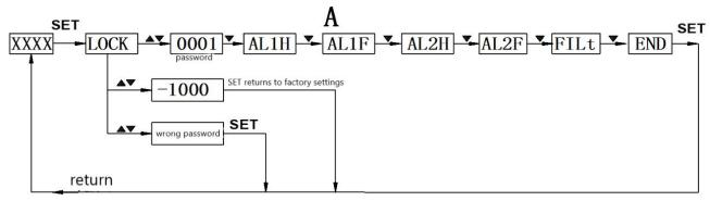
AL1H is the pull-in value of switch 1,AL1F is the release value of switch 1 AL2H is the pull-in value of switch 2, AL2F is the release value of switch 2 FILt this value is the display filter coefficient to prevent the display from jumping due to pressure fluctuation. The larger the filtering coefficient is, the more stable the display is, but the more lagged it is. 3 ~ 10 options END save exit
