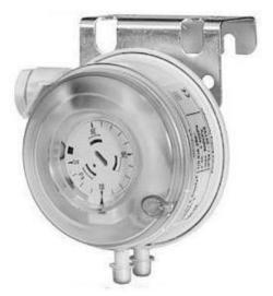
WM1204A Air Differential Pressure Switch can be used to measure the pressure difference, vacuum or air flow of non corrosive gas and output NC+NO switch control. It is featured a wholly mechanical structure which is reliable and flexible in use.
