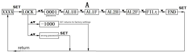
AL1H is the pull-in value of switch 1,AL1F is the release value of switch 1 AL2H is the pull-in value of switch 2, AL2F is the release value of switch 2 FILt this value is the display filter coefficient to prevent the display from jumping due to pressure fluctuation. The larger the filtering coefficient is, the more stable the display is, but the more lagged it is. 3 ~ 10 options
